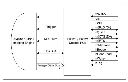
Figure 16. IS4920 / IS4921 System Architecture
